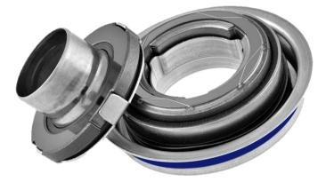
The GlideX<sup>tm</sup> - WPS for automotive water pumps is a further development of the well-known and widely applied EKK compact seal. The textured seal which ensures extremely low torque and superior sealing performance. Its non-contacting sealing under rotation provides low torque with improved wear resistance. The torque reduction is more than 90% compared to the conventional mechanical seal.
